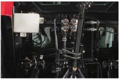
**IMPRESSIVE HYDRAULICS** A completely new hydraulic system delivers 5,500 lbs. of lift capacity and 17 GPM of implement pump flow to power all of your implements quickly and efficiently. An optional multi-coupler kit allows all loader hoses to be connected at once with a snap.
