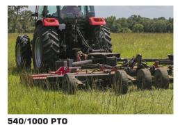
With up to 82 PTO HP (depending on model) and featuring a standard dry sump, you'll be ready for a wide range of implements to help boost productivity while reducing down time.
