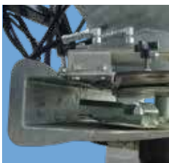
Hydraulic Shut-Off Gate
